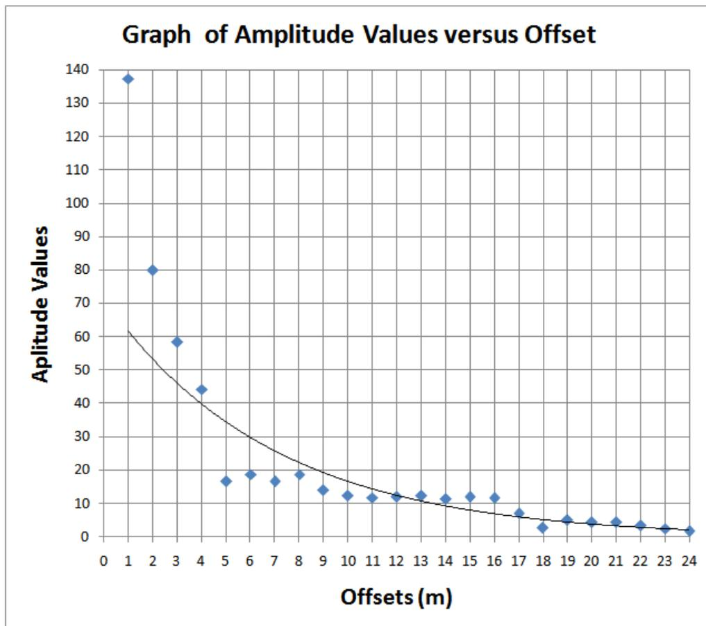
**Figure 16: Plot of the trace amplitude within a shot against the offset**
