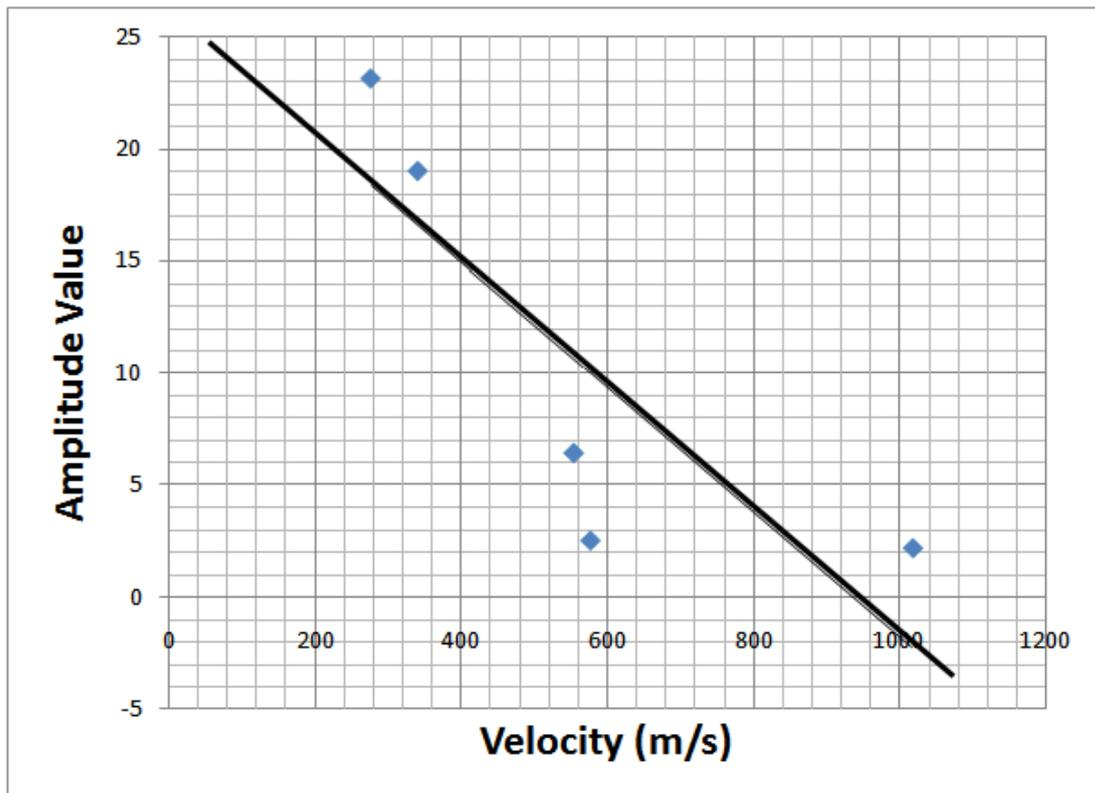
**Figure 13: Plot of extracted average Vs values and trace amplitude Values**
