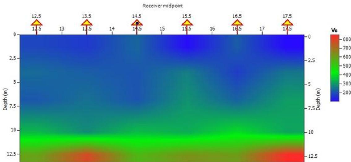
Figure 9:  $V_s$  model of profile 2, showing the distribution of shear wave velocity
