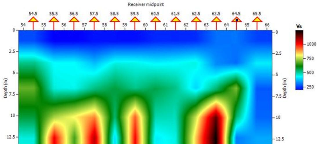
**Figure 11: Vs model of profile 4, showing the distribution of shear wave velocity**
