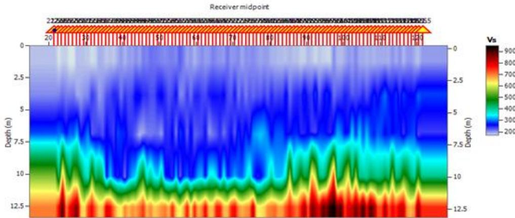
Figure 8:  $V_s$  model of profile 1, showing the distribution of shear wave velocity
