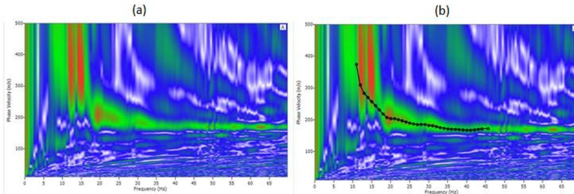
**Figure 2: (a)The generated dispersion image of a shot point (b) Extracted Dispersion**
