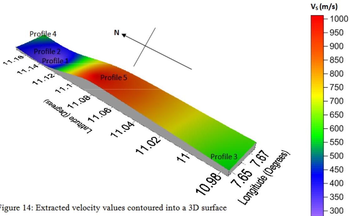
Figure 14: Extracted velocity values contoured into a 3D surface
