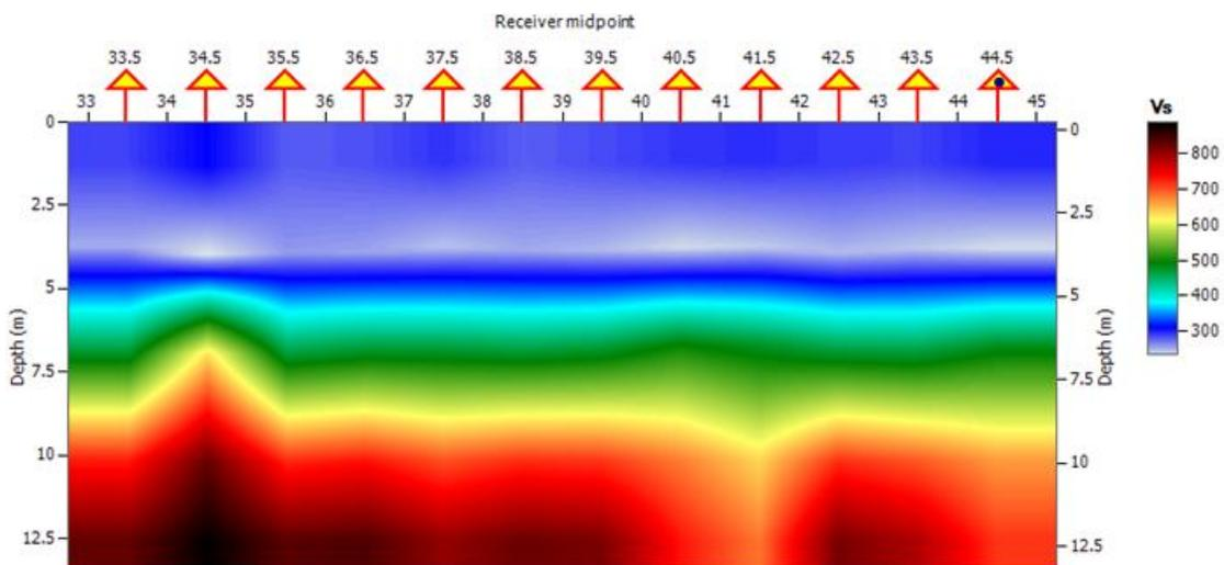
Figure 10:  $V_s$  model of profile 3, showing the distribution of shear wave velocity
