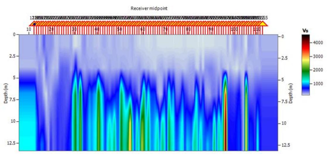
**Figure 12: Vs model of profile 5, showing the distribution of shear wave velocity**
